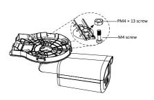
Figure 2-14 Secure Camera to Wall Mount Cover
