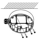
Figure 2-26 Secure Junction Box Body
