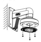
Figure 2-29 Fix Installation Plate
