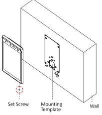
2 Fix the mounting plate to the wall with 4 supplied screws.
