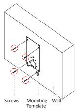
Paste the mounting template on the wall according to the 1 installation requirements. Drill holes acording to the template. Insert the expansion bolts into the screw holes.
