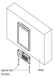
Fix the device to the mounting plate and fix the device with the set screws.
