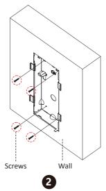
Install the gang box into the wall. a. Insert the gang box into the installation hole. Mark the gang box marker, and take out the gang box. b. Drill 4 screw holes according to the marks on the wall, and insert the expansion sleeves into the screw holes. c. Fix the gang box with 4 screws.
