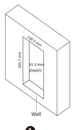
Cave an installation hole on the wall. Pull the cable out from the wall.
