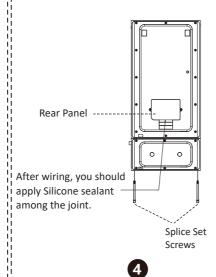
Fix the sub module to the door station with 2 set screws. Wire the device and cover the rear panel with 2 screws.
