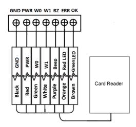
Figure 3-5 Wiring for Wiegand Communication Mode
