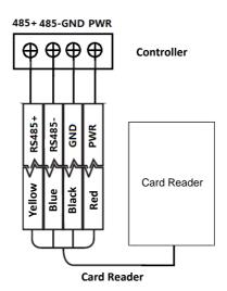
Figure 3-4 Wiring for RS-485 Communication Mode
